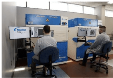
2D and 3D Radiological Inspection
