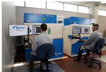
2D and 3D Radiological Inspection
