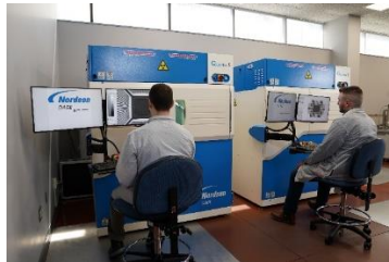
2D and 3D Radiological Inspection
